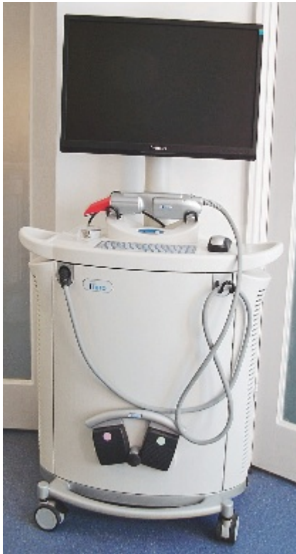
Fig 15-4a Using the intraoral digital scanner will reduce the need for impression taking using trays and impression material. Once the dentist has been trained in using the scanner to record the prepared teeth, this will improve accuracy and speed. The scanner transfers the information via the internet directly to the dental laboratory in order to save time. The picture shows the Cadent iTero scanner (Cadent, Carlstadt, NJ).
